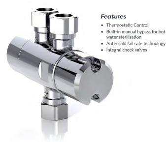
Inta's thermostatic mixing valve comes equipped with its own unique by-pass device to sterilise the valve and the waterway up to the tap without having to be disassembled. Whilst also delivering safe, blended hot water to taps, showers, bidets and other water outlets.
